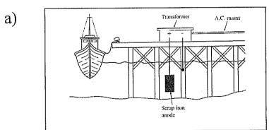
Run a current through the scrap iron, making it the anode.
