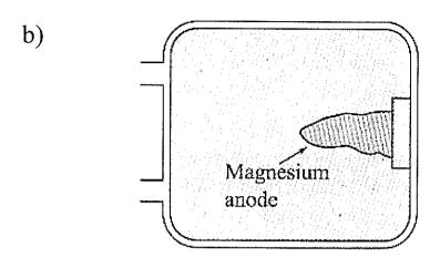
Use a sacrificial anode, by electrically connecting a more reactive metal which oxidises in preference to iron.
