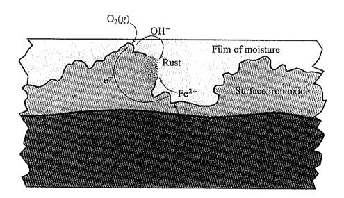
This can also occur in areas where the iron is protected from oxygen by being sealed. This is called the differential aeration principle.
