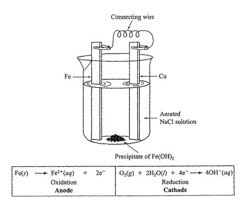
In the presence of water, iron reacts to form green iron (II) hydroxide which slowly further reacts to give the brown iron (III) hydroxide which can further partially
